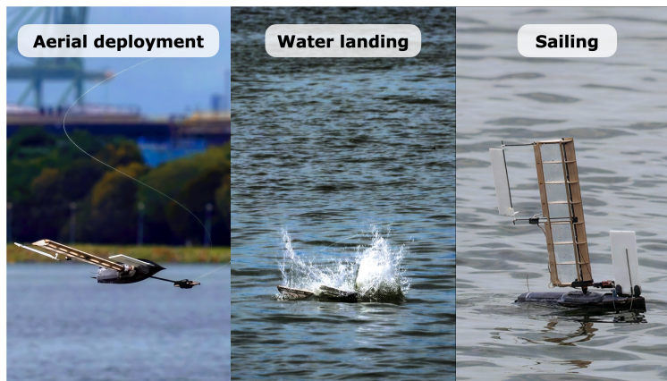
Movie 1: Aerial deployment and hybrid operation of ALBATROSS. This video shows the real-world aerial deployment, autorotation and sailing operation of ALBATROSS.
